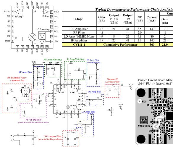
Printed Circuit Board Material: .014" FR-4, 4 layers, .062" total thickness
